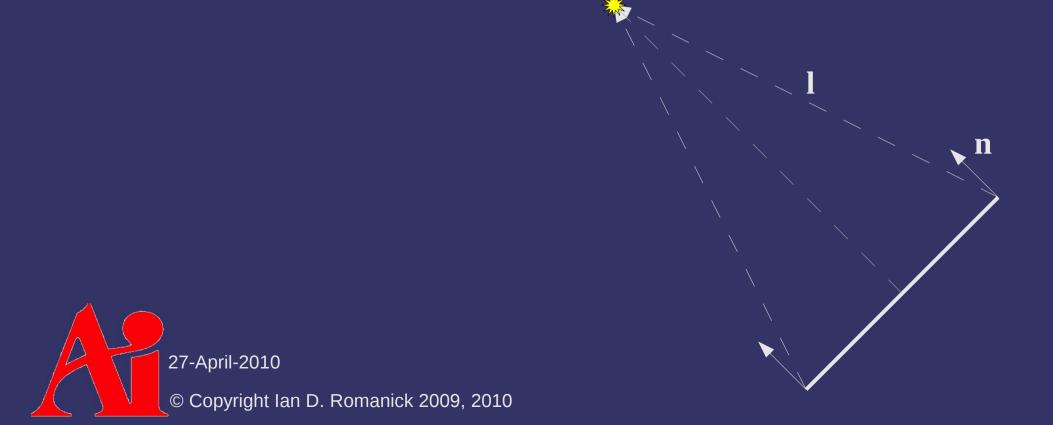
Calculate the I vector by subtracting the vertex position from the light position and normalize the result
